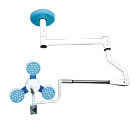
1.00.000 Lux Intensity 100 - 150 mm Spot Diameter Depth Illumination 10 - 15 cm · Colour Temp. 4000 - 4850 K 91 Ra Colour Rendering Index: Focusing Manual LED Average Life >50000 Hrs Number of LED 57 Diameter of Light : 580mm Intensity Control 10~100 Digital Power Supply 220V/50Hz AC : 40 X 2 Watt **Power Consumption**  Special Function Memory
