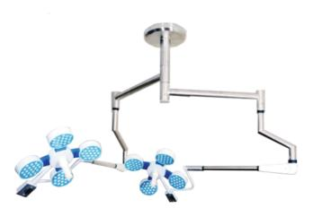
1,25,000 Lux Intensity Intensity Satellite 1,25,000 Lux Spot Diameter 100 - 150 mm 10 - 15 cm **Depth Illumination** Colour Temp. 4000 - 4850 K Colour Rendering Index : 91 Ra Focusing Manual >50000 Hrs LED Average Life Number of LED 76 X 2 Diameter of Light 580mm X 2 10~100 Digital Intensity Control Power Supply 220V/50Hz AC Power Consumption 40 X 2 Watt Special Function Memory
